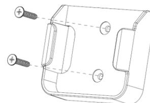
Installation of transmitter wall mount holder with two screws.
