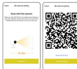
8. Once connected to your home WiFi, scan the 'QR Code' with smart camera. Hold 'QR Code' approx. 20 cm in front, facing the smart doorbell camera lens.
