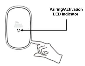
2. Press the Bell Press once, the LED indicator light on the Chime/Receiver will go Off, and the pairing will be complete
