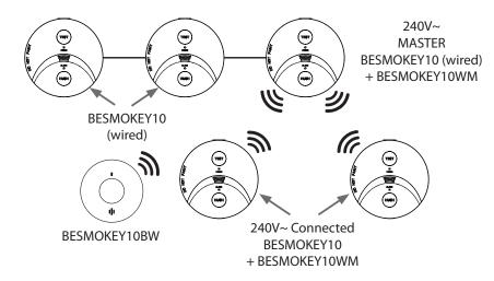
BESMOKEYREM can be installed on wireless network for convenient control.
