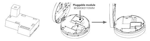
To make wireless, before removing battery tag add BEMOKEY10MW, then connect battery and power. Follow instruction to pair the wireless alarms in the network.
