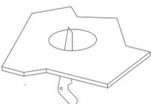
1. Open a hole according to the cutout size of led downlight.
