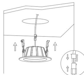
3. Connect the downlight with driver, hold back the spring clip then push the downlight into the hole.
