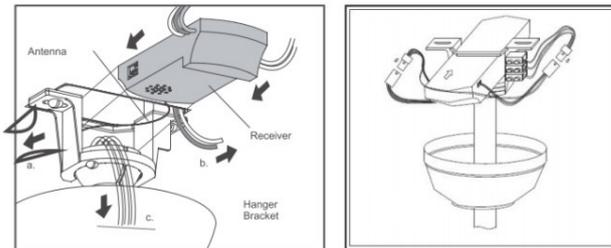
Make the wiring connection as shown in the picture. Ensure that the DIP switches on the receiver and transmitter are set to the same positions.
