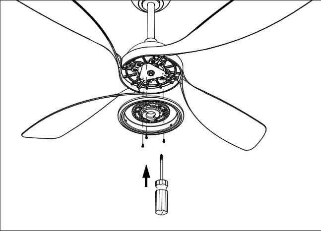
Install the LED light plate onto the steel bracket as illustrated with the 3 supplied screws.
