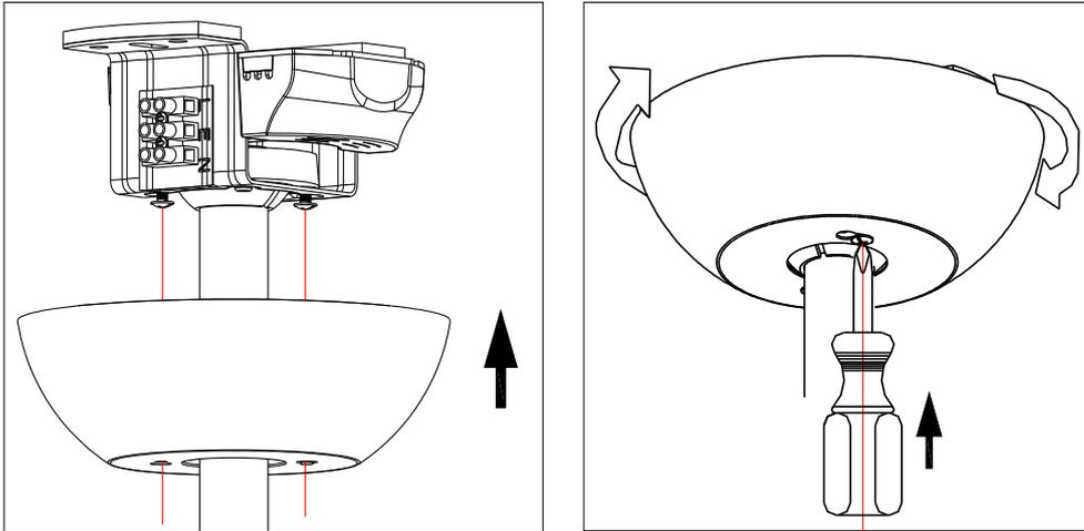
Carefully put the screw cap on using the piece of magnetic supplied.
