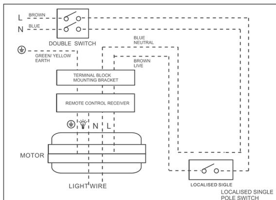
**Step 1:** Connect the EARTH wire to the terminal port marked “⊕” on the terminal block mounting bracket.
