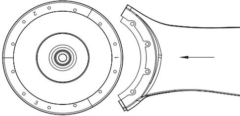
To install align the blades with the orifice as shown.
