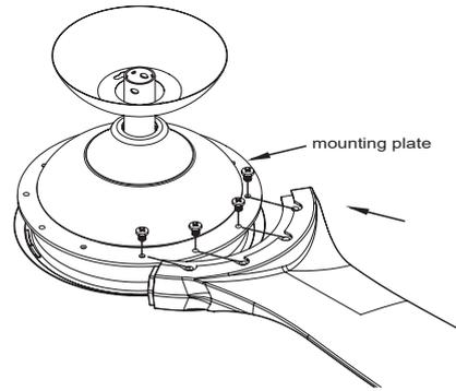
Attach the blade to the top of the motor using the 4 blade screws provided. Tighten the screws and repeat this procedure for all blades.
