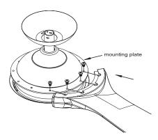
Attach the blade to the top of the motor using the 4 blade screws provided. Tighten the screws and repeat this procedure for all blades.
