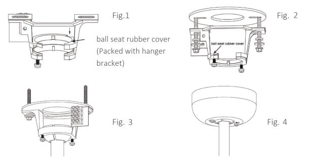
The inside canopy cover ring (1) has two keyhole slots that allow it to be mounted onto the screw heads on the two protruding screws from the mounting bracket. Slide the canopy cover ring up the downrod, and allow the two protruding screw heads from the mounting bracket to go into the keyhole slots on the canopy cover ring. Once engaged, twist the canopy cover ring to lock it onto the screw heads.(Fig.4a)
