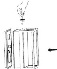
Attach fitting back onto the bracket using the allen key supplied.
