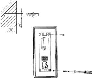
Mount the bracket on the desired surface using the two screws supplied.
