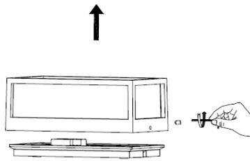
Unscrew and remove the mounting bracket using the allen key supplied.
