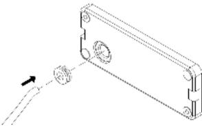
Fit main cable and the silicon cover through the entry at the back.
