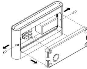
Remove mounting bracket by the Allen Key.
