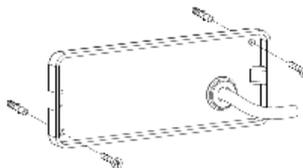
Drill holes and mount the bracket on desired surface.
