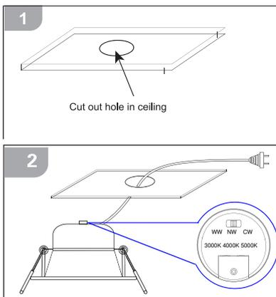
1 Cut out (size:90mm) hole in the ceiling. Ensure there is sufficient clearance in the area where you will position the fitting.
