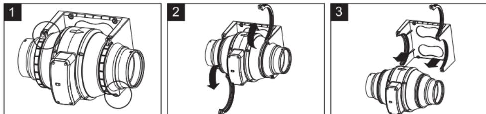
2. Secure the mounting bracket fan flange assembly to a fixed structure.
