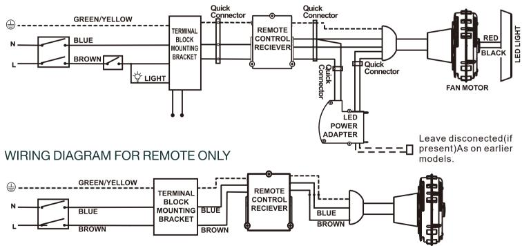
WARNING: For your safety, ensure the mains supply is switched OFF to the wiring circuit before performing any electrical wiring tasks. MAKE THE WIRING CONNECTION AS SHOWN IN THE APPROPRIATE IMAGE.
